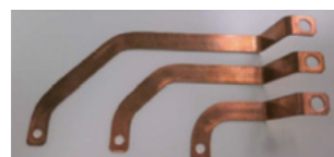
Bus bars produced with a forming machine
